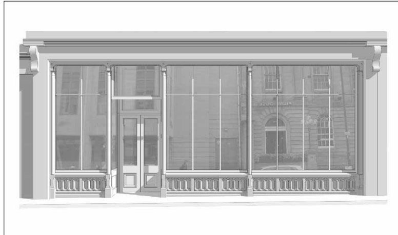
Design proposal reinstating cast iron shopfront
