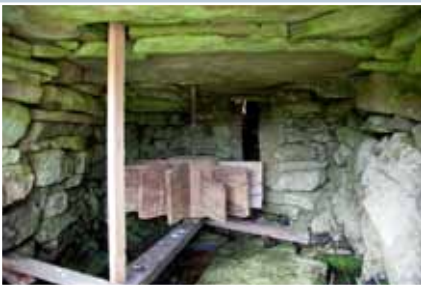
A repaired later 19th-century horizontal waterwheel, part of a corn mill in a series of nine such mills at Troswick, Shetland. © N Haynes.
