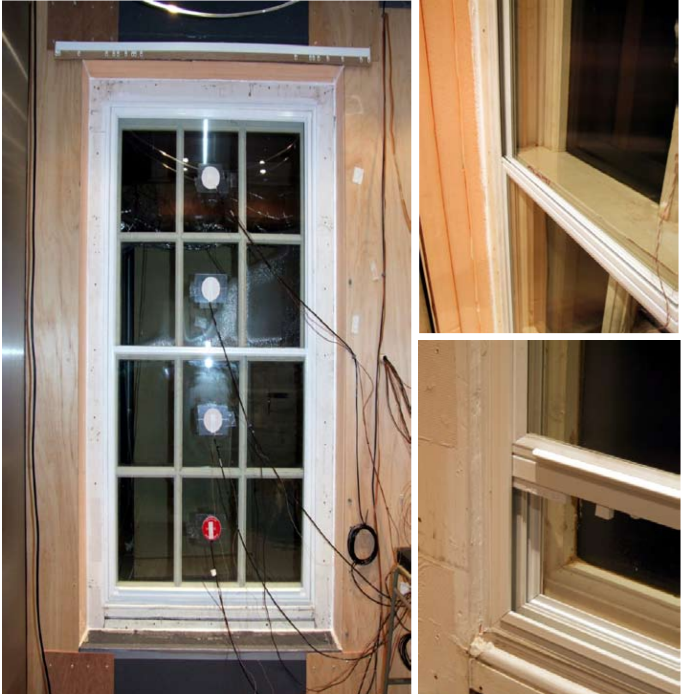
Figure 11: Secondary glazing system
