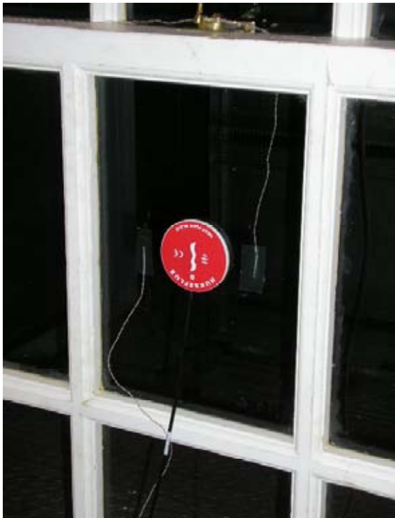
Figure 13: Heat flux sensor in position on glazing and sensor dimensions
