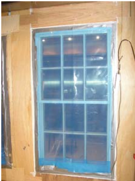
Figure 19: The window covered with air impermeable polythene sheet to determine background air leakage of room.
